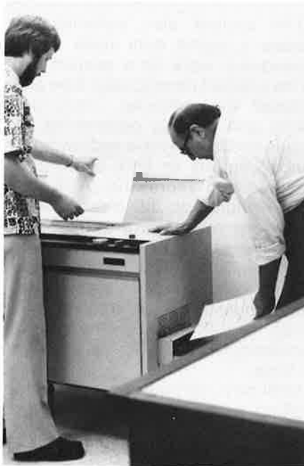
Reduced-scale modules are quantity-reproduced on a Royal Bond RBC 1 copier. The Royal can also produce reverse-reading and sticky-back transparencies for applying notes, details, etc. to a reproducible vellum or sepia Mylar, thus saving much drafting time.
