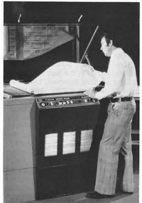
To produce a sepia Mylar film, an opaque sheet (with elements from the Design Master camera and 695 copier) is put together with blank sepia Mylar film. It is exposed on the NuArc Flip Top 46 UP, creating a sepia Mylar film, which is then processed through a diazo machine.
