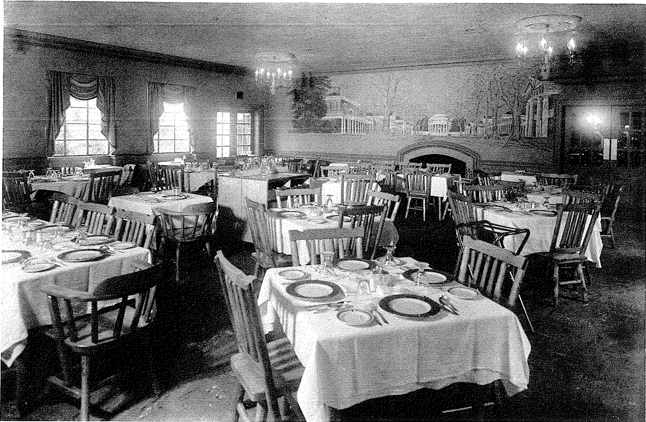
A view in the dining room of Thomas Jefferson Inn. The wood trim is green, and the plaster has an ashes-of-roses color. The mural depicts the University of Virginia. Air-conditioning inlets are made an integral part of the light fixtures, and the fireplace serves as a return duct for the air-conditioning unit.
